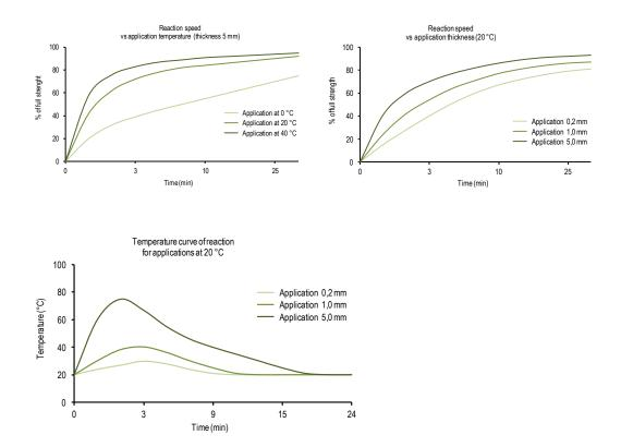
TECHNICAL CHARACTERISTICS OF CURED PRODUCT The below properties have been measured through standard samples tests, made bonding by overlapping samples of different materials of dimensions  $100 \times 20 \times 20$  mm with an adhesion area of  $20 \times 20$  mm.
