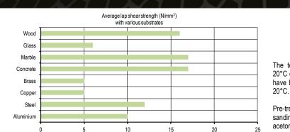
The tests have been conducted at  $20^{\circ}$ C on metal to metal joints, which have been hardened for 48 hours at  $20^{\circ}$ C.
